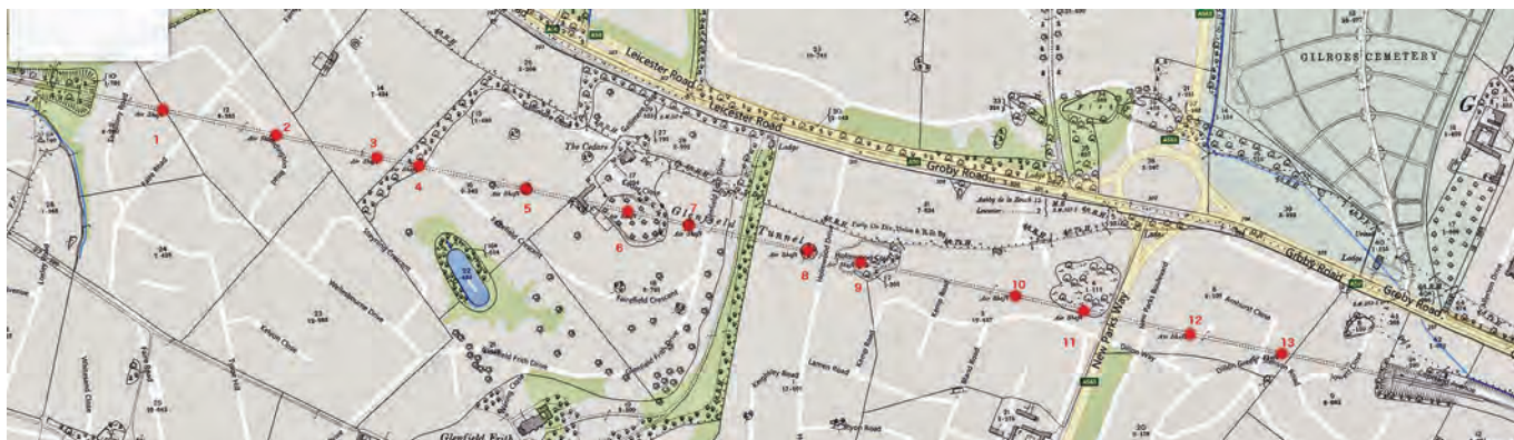
Glenfield tunnel overlaid onto a modern map. The 13 ventilation shafts are shown
